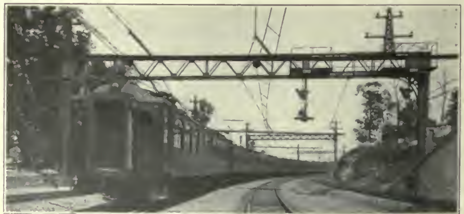
FIG. 541. MULTIPLE-UNIT TRAINS. Motor Car Train for 11,000-Volt Single-Phase Overhead Contact Operation, New York, Westchester & Boston Railway.
